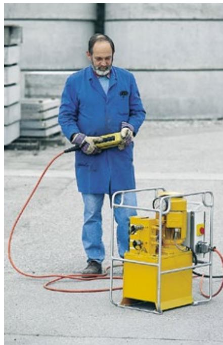
Hydraulic Pump with a Remote Control
